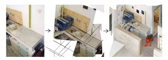
Image 8. Remaking a photograph as an axonometric projection
