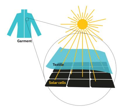
↑ The solar cell, underneath the surface fabric of a jacket, can produce enough energy for powering wearable devices.
